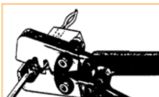
3. Put terminal in crimping tool, then position wire and seal in place.
