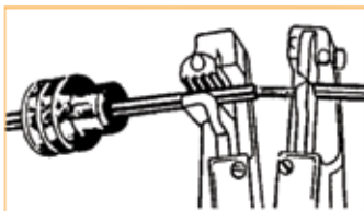
1. Apply seal to cable, before stripping insulation.
