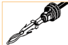
4. Crimp and visually inspect for a good crimp before installing in connector body.
